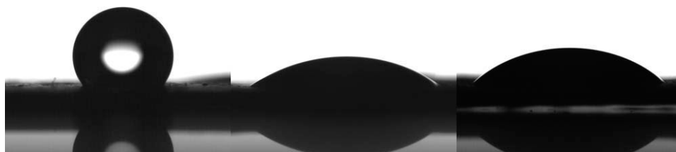
Figure 5 Images of contact angle measurements on electrospun PCL nonwoven (left), sPEEGE/PCL (15 : 85) (middle) and sPEEGE/PCL (25 : 75) (right) nonwovens.
